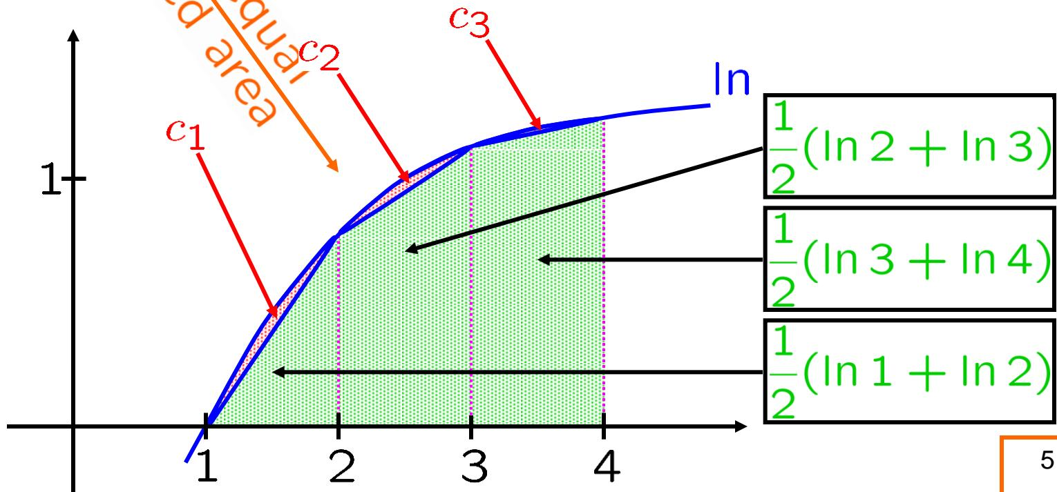
$$\int_1^4 \ln x \, dx = \ln 1 + \ln 2 + \ln 3 + \ln 4 - \frac{\ln 4}{2} + c_1 + c_2 + c_3$$
