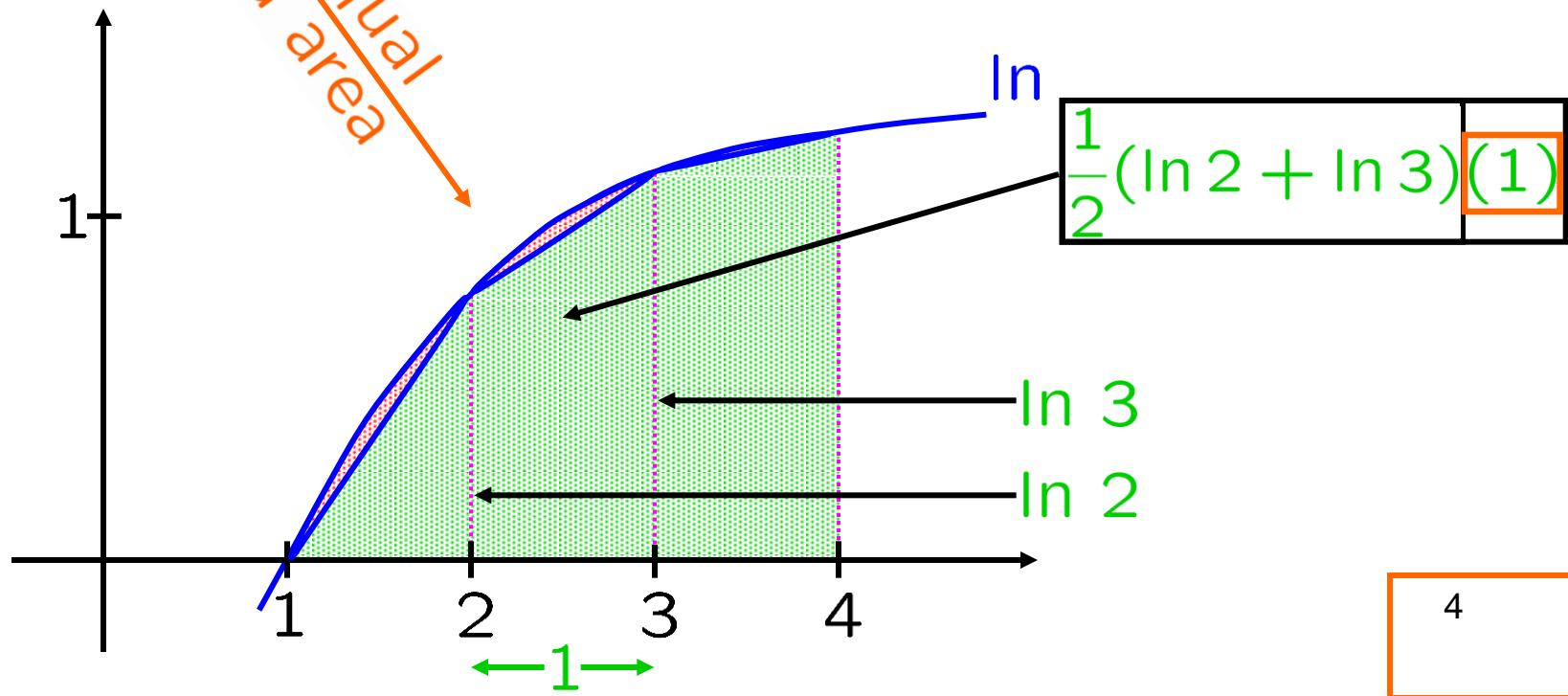
$$\int_1^4 \ln x \, dx \approx \frac{1}{2}(\ln 1 + \ln 2) + \frac{1}{2}(\ln 2 + \ln 3) + \frac{1}{2}(\ln 3 + \ln 4) + c_1 + c_2 + c_3$$
