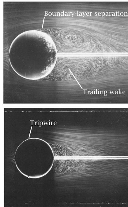
**Figure 4** Flow past a smooth sphere, clearly exhibiting boundary-layer separation and the resulting trailing wake. A tripwire has been added to the lower sphere. The resulting turbulence in the boundary layer delays separation and so leads to a smaller trailing wake. (Photos from *An Album of Fluid Motion*, Milton Van Dyke.)
