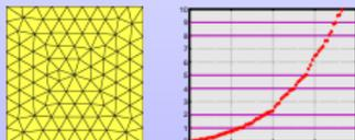
On this structured mesh the discrete eigenvalues converge to the true eigenvalues, but also to a sequence of spurious ones.
