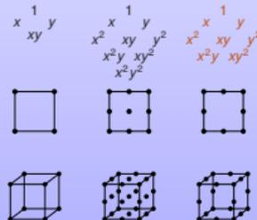
For distorted quads or hexes, we use a multilinear map from a reference cube, and compose to get the shape functions.
