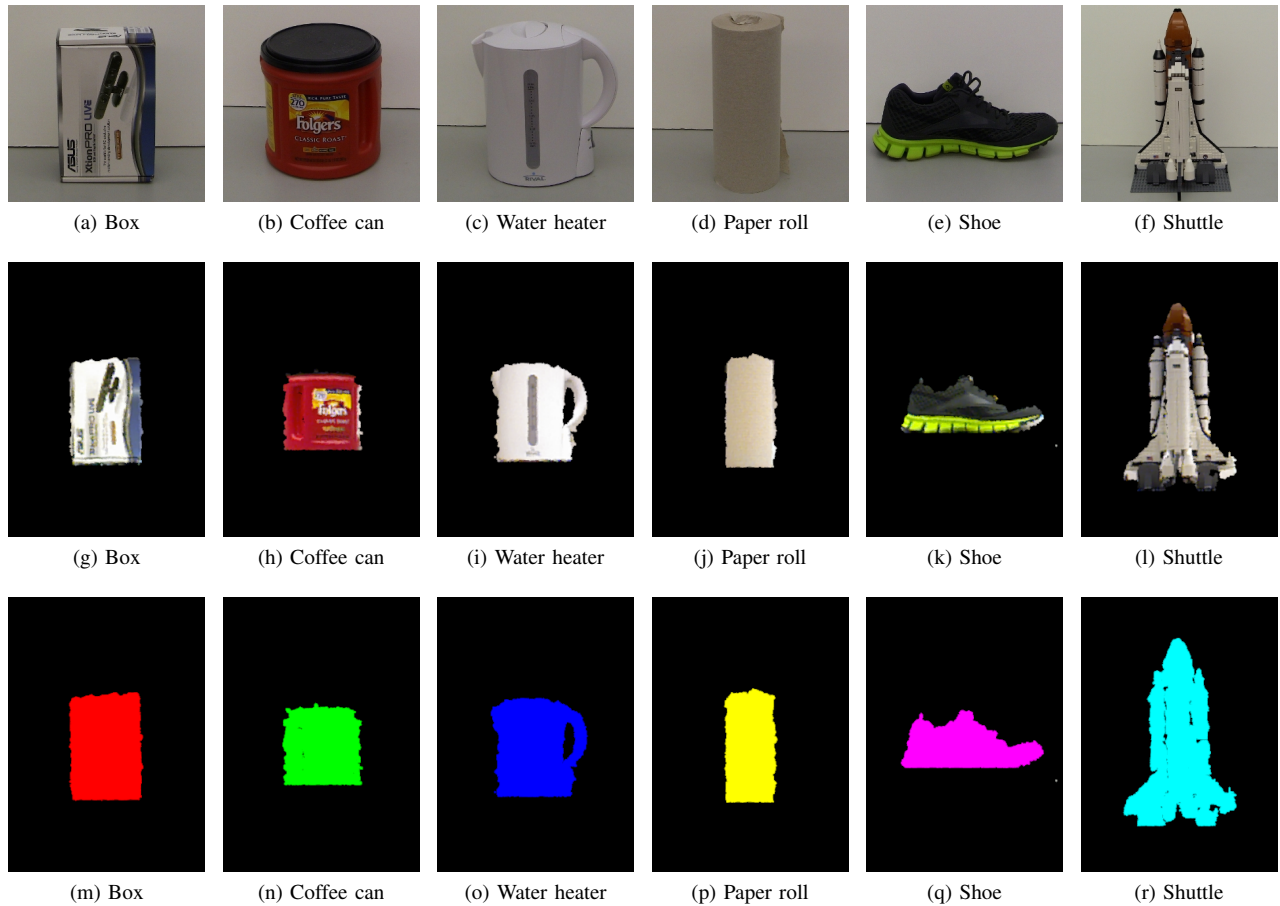
Fig. 3: These figures show the different objects used in the experiment. The top row gives an RGB view of the objects, the middle row depicts the robot’s view of the object, and the bottom row gives the color coding corresponding to each object.
