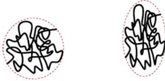
FIGURE 1. Representation of the step-length tensor L : isotropic polymer (left) and nematic polymer (right).
