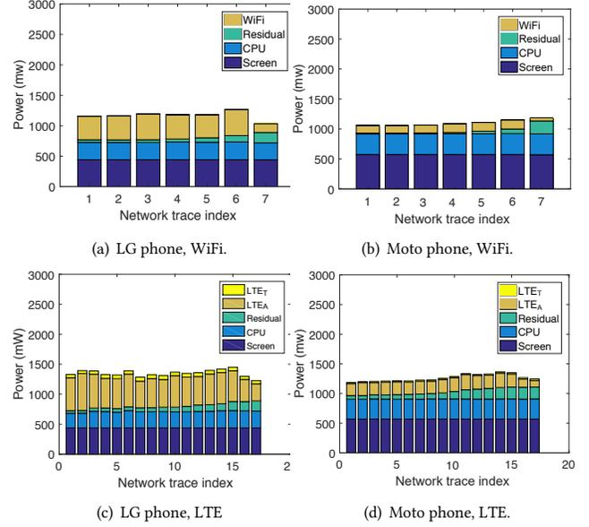
Figure 9: Power breakdown of ABR streaming for a regular video (Animation) in WiFi and LTE networks.
