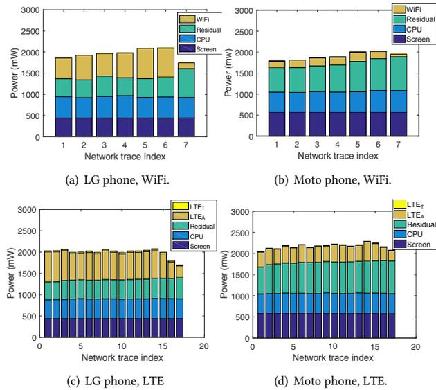
**Figure 11: Power breakdown of ABR streaming for a 360° video (Sci-Fi) over WiFi and LTE networks.**
