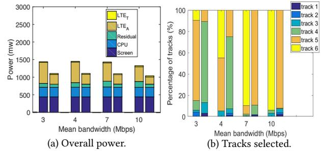
**Figure 13: Energy saving by per-segment track reduction (LG phone). For each setting, the two bars represent the result of the original scheme and that after applying the strategy.**
