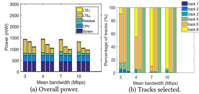
**Figure 12: Energy saving by capping the top track (LG phone). For each setting, the three bars represent the results for not capping, and capping to 720p and 480p, respectively.**
