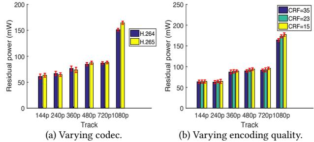
Figure 3: Impact of codec and encoding quality (LG phone).
