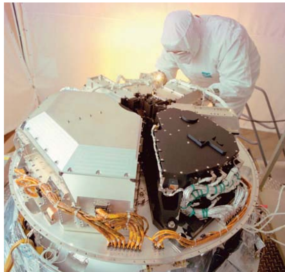
FIG. 9. (Color) The Spitzer family portrait: the science instruments mounted on the multiple instrument chamber baseplate at Ball Aerospace during cryogenic telescope assembly integration and testing. Clockwise from the lower right are IRAC (in black), MIPS, IRS long-low, IRS long-high, IRS short-low, and IRS short-high. Courtesy of NASA/JPL-Caltech.
