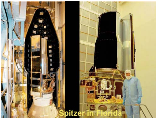
FIG. 32. (Color) Spitzer during installation on the rocket at Kennedy Space Flight Center. The left hand picture shows the radiative side of the observatory and the right hand picture shows the Sunward side with the observatory mounted in the nose cone of the Delta rocket. Michael Werner is shown for scale. Courtesy of NASA/JPL-Caltech.
