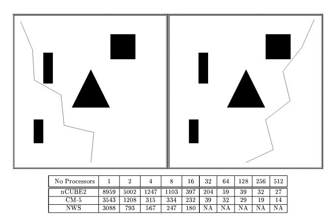
Figure 6: Start and Goal Configurations for Six Degree of Freedom Robot operating in a  $256 \times 256$  cell workspace. Each C-space axis (joint) has 256 possible discrete positions. The base of the robot is fixed in the bottom-center in each frame of the picture. The table summarizes the data for runs on different multicomputers. All times are in seconds.
