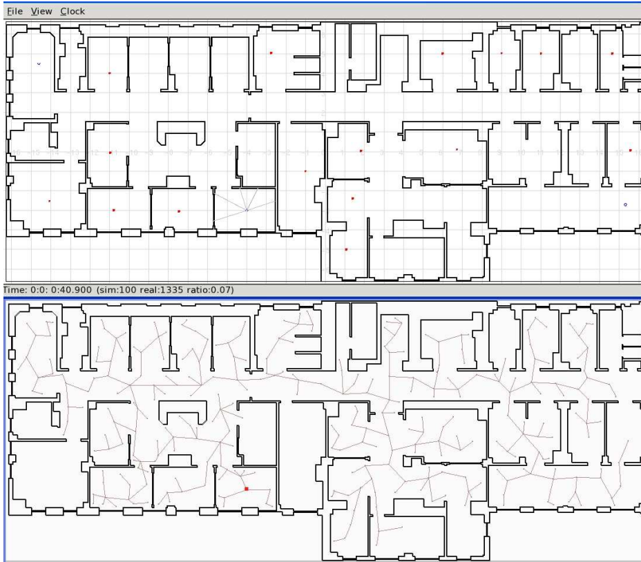
Figure 2. The hospital environment. The top part of the figure shows the Stage simulation, with the locations of the tasks and of the robots. (The active robot has its range sensor traces shown). The lower part shows the paths generated by the RRT algorithm, with the location of the active robot on the paths indicated by a square. This is one of the single robot experimental runs, where only one robot is active.
