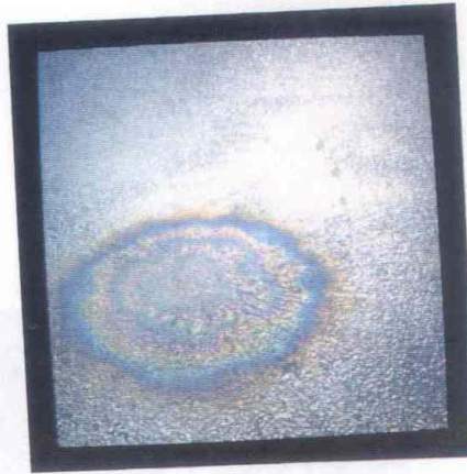
Fig. 5: Simulation of the interference colors produced by an oil slick on wet asphalt pavement.
