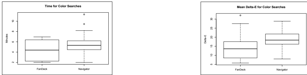
Figure 8. Box and whisker plots of the 5 number summary statistics (minimum, first quartile, median, third quartile and maximum) for completion times (left) and accuracies (right) in the first study. The circles are outliers and are beyond 1.5 times the inner quartile range.
