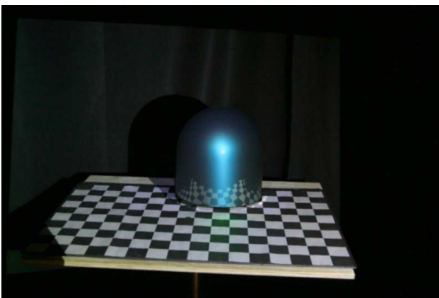
Figure 4. Environment mapping is added to make the shape shown in Figure 3 appear glossy
