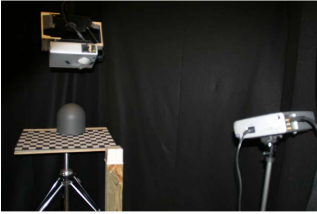
Figure 6. The final system setup: a color simulation projector (left), magnetic tracker (middle), and projector light source (right).
