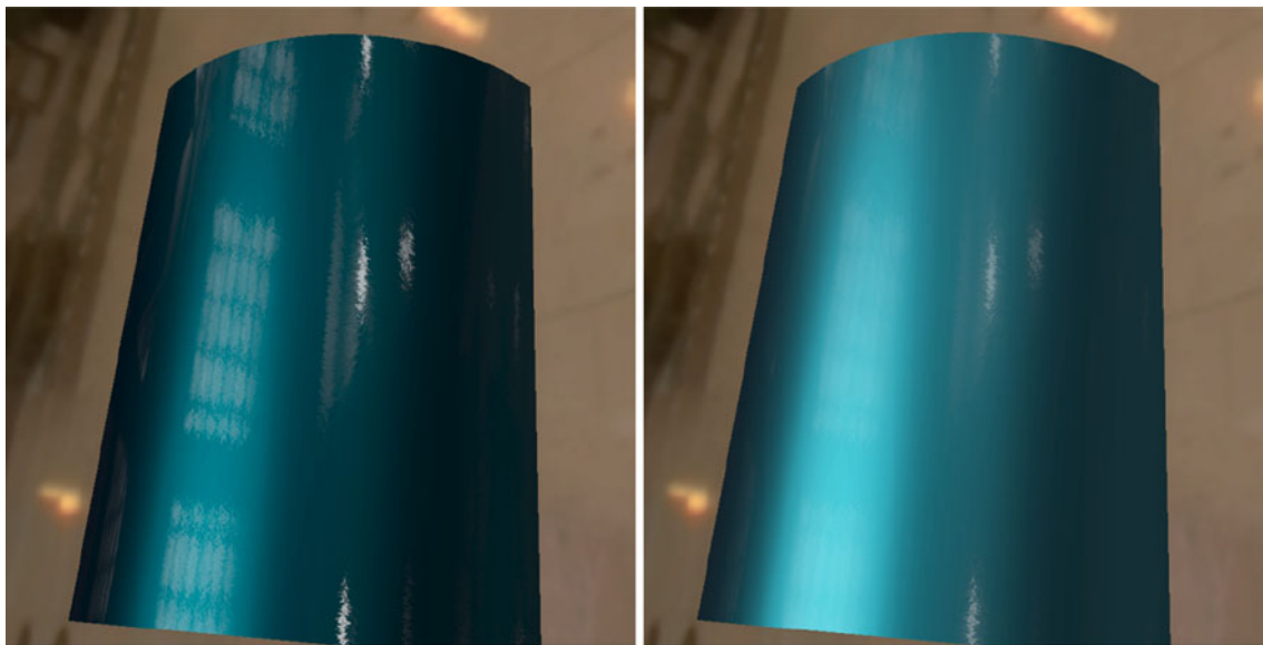
Fig. 8: Two images produced by the rendering system. On the left is an image of orange peel on metallic dark blue paint. On the right is the same orange peel on a less glossy sample of light blue paint; this makes the orange peel less noticeable
