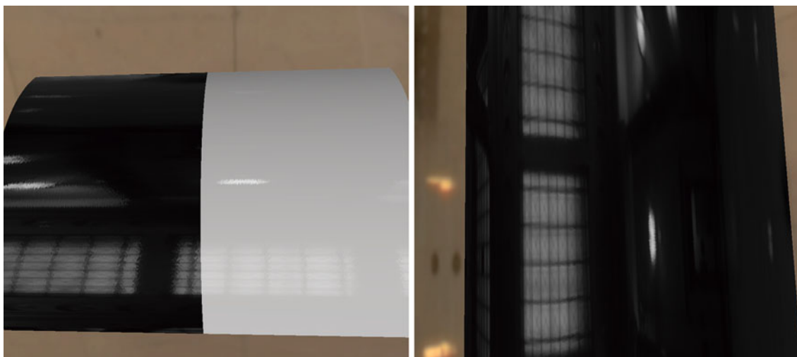
Fig. 11: Two images from the second orange peel experiment. Left: An image with differing lightness and orange peel values. Right: One of the control images with varying orange peel values but the same lightness
