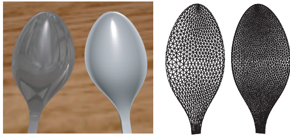
Figure 9: Reflections produce a masking pattern and reduce the number of polygons required in the mesh. The shiny teapoon on the left has only 1027 vertices, and the diffuse teapoon on the right has 2761 vertices.
