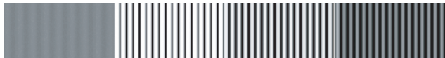
Figure 3. A sine wave and its visibility map at viewing distance 1, 2, and 3 meters.
