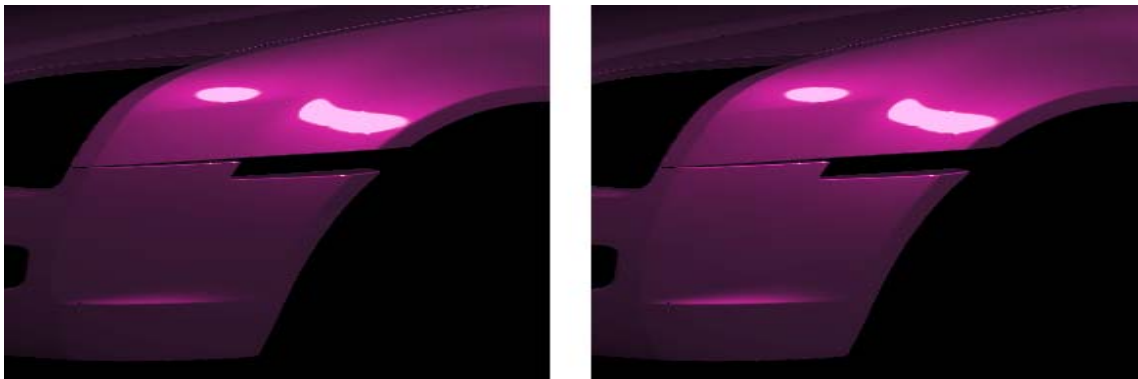
Figure 5: Bumper and fender misaligned by 8 degrees. Identical metallic paints cause a color mismatch (left) while painting the bumper a different color, determined using the inverse trompe l'oeil technique, eliminates the problem (right).
