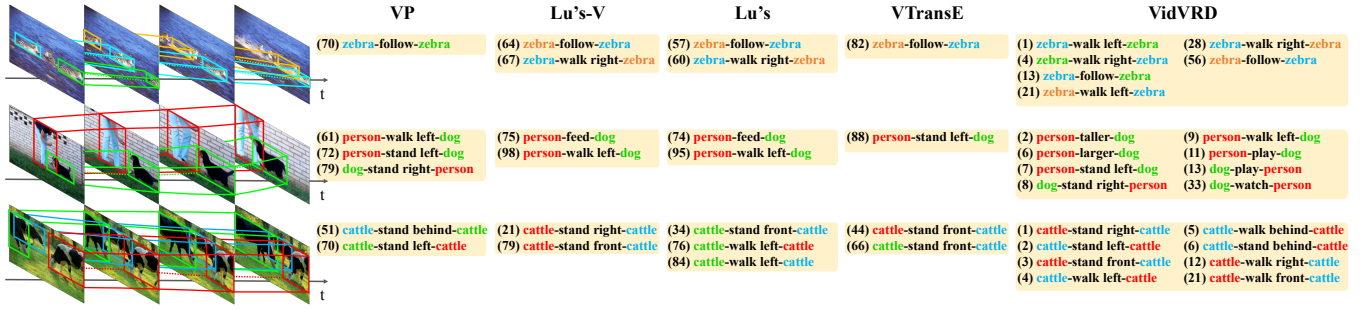
Figure 5: Qualitative examples of visual relation detection using different methods. The correct visual relation instances in the top 100 results are shown, and their ranks are marked in front of them with parentheses. Note that the object localization results are not shown due to space limitation, but they are all required to have sufficiently high vIoUs to the ground truth object trajectories, which are shown on the video frames with different colors.
