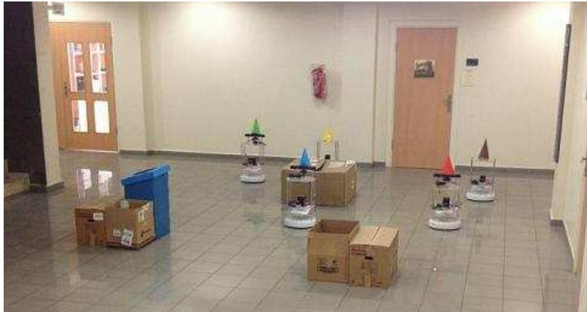
Figure 1.1. A multi-robot system of 5 robots in an environment with a variety of obstacles.
