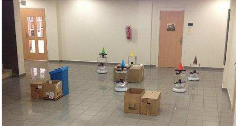
Figure 4.5. The experimental setup of a patrolling mission. It is assumed that as robots start moving around, they encounter dynamic and cooperative tasks which they need to handle.
