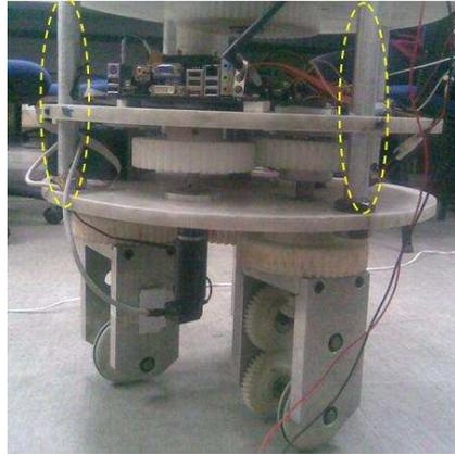
Figure C.3. Aluminum pipes connecting the planes.
