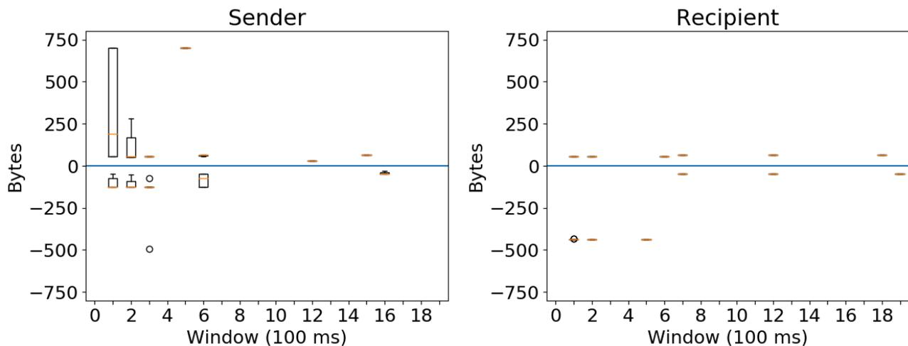
Figure 7: Network traffic pattern for sending and receiving Signal messages.
