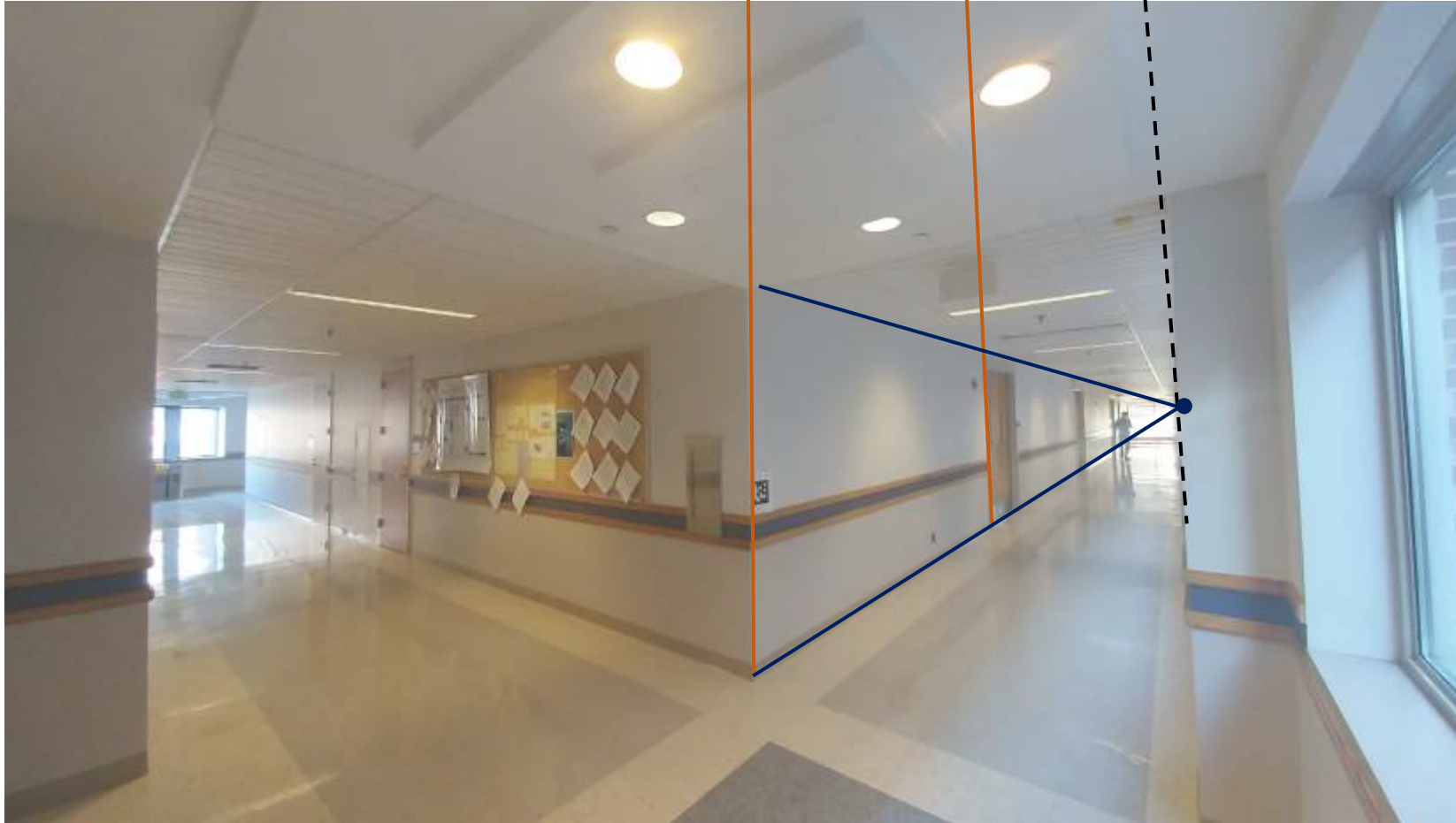
Different plane produces different vanishing line.
