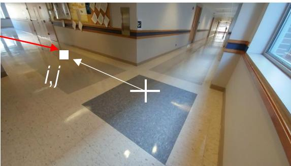
$$f = f_m \frac{W_{\text{img}}}{W_{\text{ccd}}} = 0.00153 \frac{3840}{0.0048} = 1224 \text{ pix}$$
