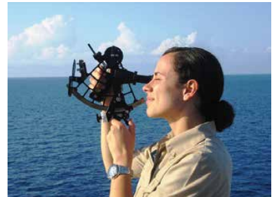
Figure 1.2: Sextant is used to measure the angle between star/moon/sun and horizon.
