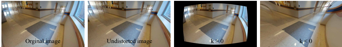
Figure 1: Lens distortion rectification.
