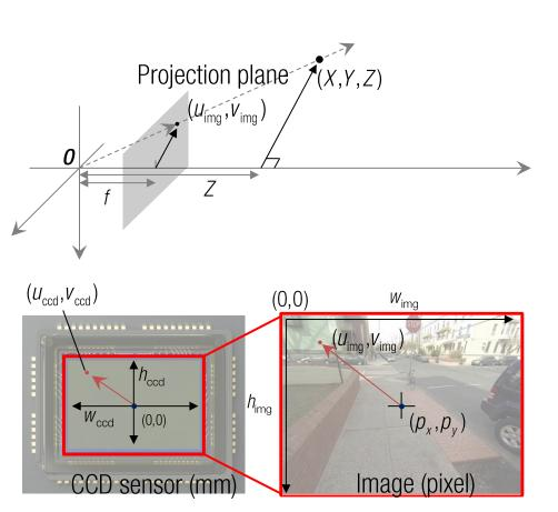
$$(u_{\text{ccd}}, v_{\text{ccd}}) = (f_{\text{m}} \frac{X}{Z}, f_{\text{m}} \frac{Y}{Z})$$
