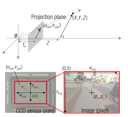
$$(u_{\text{ccd}}, v_{\text{ccd}}) = (f_{\text{m}} \frac{X}{Z}, f_{\text{m}} \frac{Y}{Z})$$
