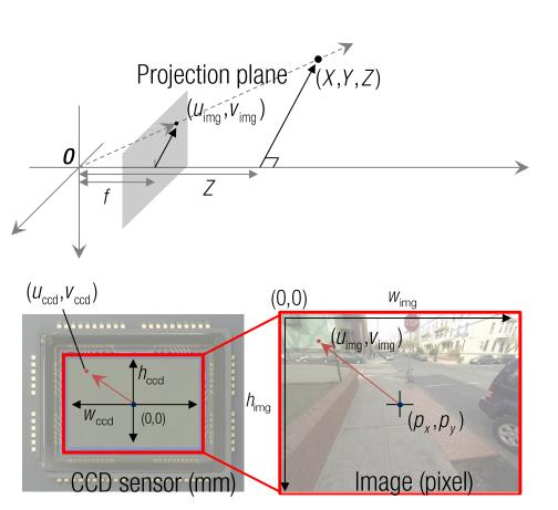
$$(u_{\text{ccd}}, v_{\text{ccd}}) = (f_{\text{m}} \frac{X}{Z}, f_{\text{m}} \frac{Y}{Z})$$
