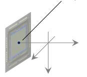
$$\frac{u_{\text{ccd}}}{W_{\text{ccd}}} = \frac{u_{\text{img}} - p_{x}}{W_{\text{img}}} \qquad \frac{v_{\text{ccd}}}{h_{\text{ccd}}} = \frac{v_{\text{img}} - p_{y}}{h_{\text{img}}}$$
