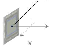
$$\frac{U_{\text{ccd}}}{W_{\text{ccd}}} = \frac{U_{\text{img}} - p_{x}}{W_{\text{img}}}$$
