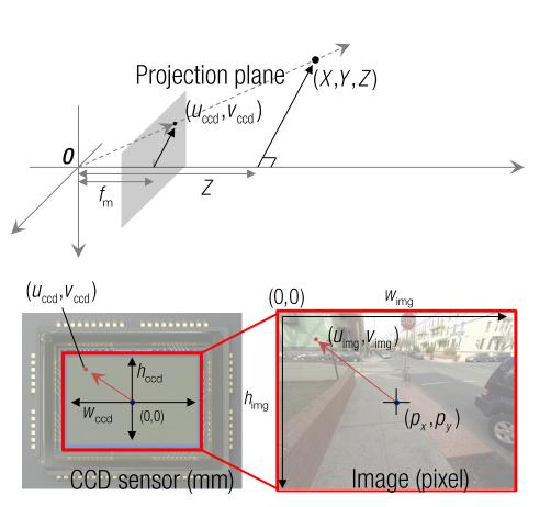
$$(u_{\text{ccd}}, v_{\text{ccd}}) = (f_{\text{m}} \frac{X}{Z}, f_{\text{m}} \frac{Y}{Z})$$
