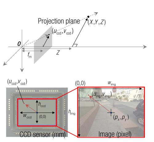
$(u_{\text{ccd}}, v_{\text{ccd}}) = (f_{\text{m}} \frac{X}{Z}, f_{\text{m}} \frac{Y}{Z})$  : Metric projection
