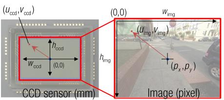
$$U_{\text{img}} = f \frac{X}{Z} + p_{x} \longrightarrow ZU_{\text{img}} = fX + p_{x}Z$$
