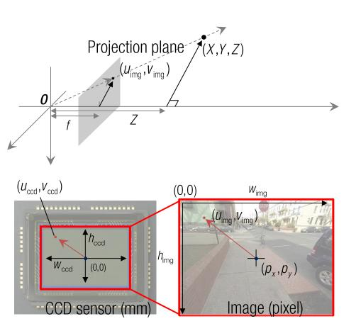
$$(u_{\text{ccd}}, v_{\text{ccd}}) = (f_{\text{m}} \frac{X}{Z}, f_{\text{m}} \frac{Y}{Z})$$
