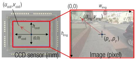
$$U_{\text{img}} = f \frac{X}{Z} + p_{x} \longrightarrow ZU_{\text{img}} = fX + p_{x}Z$$
