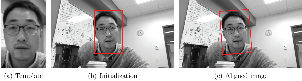
Figure 5: You will use the initial estimate of the affine transform to align (i.e., track) next image. (a) Template image from the first frame image. (b) The second frame image with the initialization of the affine transform. (c) The second frame image with the optimized affine transform using the inverse compositional image alignment.
