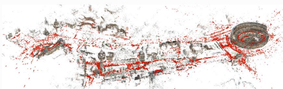
Sparse model of central Rome using 21K photos produced by COLMAP's SfM pipeline.
