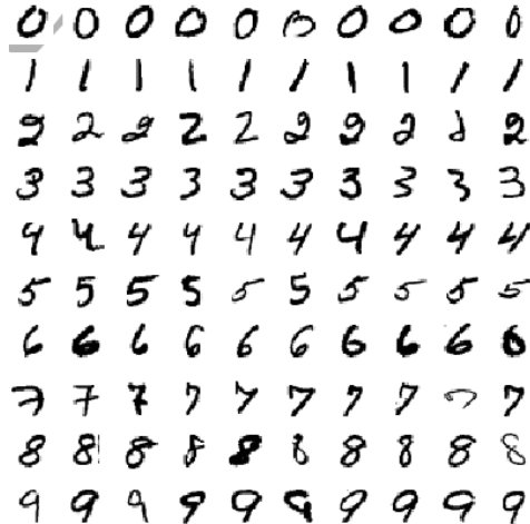
Figure 1: You will implement (1) a multi-layer perceptron (neural network) and (2) convolutional neural network to recognize hand-written digit using the MNIST dataset.
