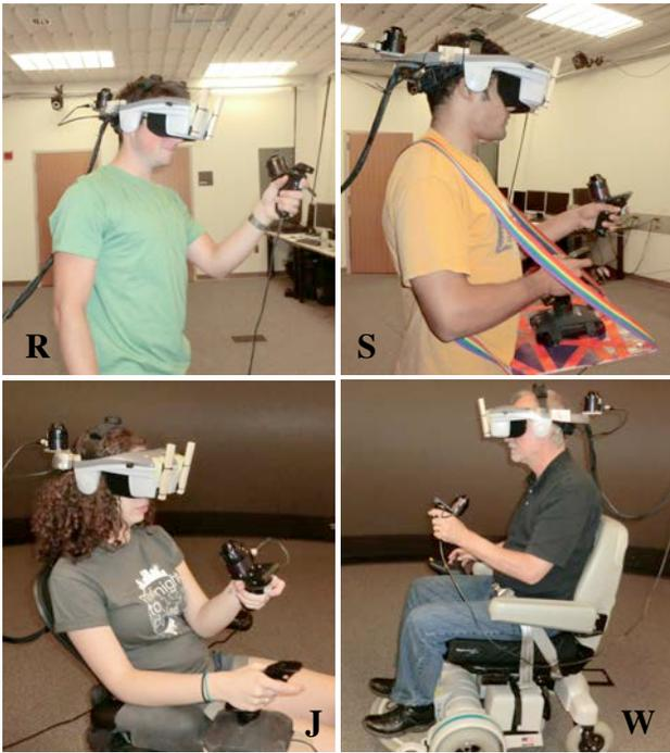
Figure 3. Photographs showing the different locomotion methods: real walking (R), joystick translation while standing (S), motorized wheelchair (W), and joystick translation while sitting (J).
