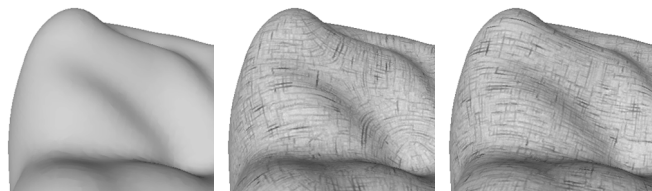
Figure 1: A close-up view of the top portion of a tooth dataset, depicted, from left to right, with: no texture, with an orthogonal texture pattern following smoothed principal directions, and with an orthogonal texture pattern following constant uniform directions in object space.
