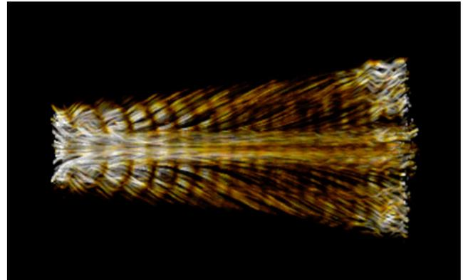
**Color Plate 3:** When streamlines are represented as a volume texture, color and opacity information can be easily redefined based on any function of the flow values across the volume. In this image, vorticity magnitude is locally mapped to streamline color using a heated-object colorscale. The striations along the axial direction reveal the presence of periodic waves propagated down the jet axis.
