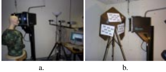
Figure 4. Experimental Setup. a) mannequin, scanner head and camera cluster. b) 3D target for coordinate frame registration.
