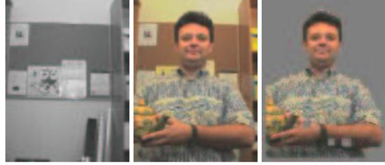
Figure 3. Background image, foreground image and subtracted result.
