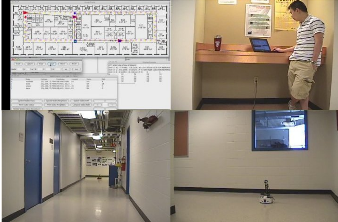
Figure 10: Known user trajectory experiment-1: Left top figure shows the implementation graphical user interface (GUI). The GUI shows the initial configuration of the robotic router system. Right top figure shows the Mac base station. Bottom left figure shows the mobile router in the middle vertical hallway. Bottom right figure shows the user which is a robot that controlled remotely by the base station.
