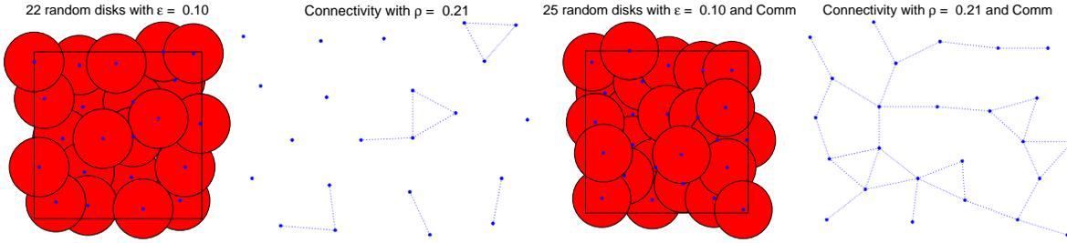
Fig. 6. Disks sampled without replacement. : **Left, Middle-left:** Even though removing already covered regions from the sampling domain results in fewer sensors, it also causes loss of connectivity. **Middle-right, Right:** Algorithm *SampleWithoutReplacementwithComm* ensures connectivity.
