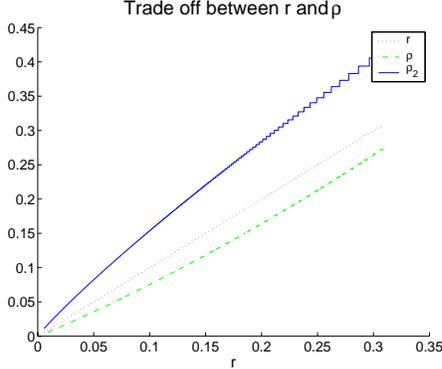
Fig. 5. The trade-off between the sensing range  $r$  and communication range  $\rho$ : For a given  $r$  value,  $\rho$  is obtained by using  $n = \frac{d}{\varepsilon} \log \frac{d}{\varepsilon}$  in Theorem 4 and  $\rho_2$  was obtained by  $n = \frac{d}{\varepsilon}$  with  $\varepsilon = \pi r^2$ .
