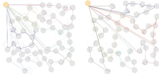
Fig. 9. **Left:** Data gathering using an area-based partitioning approach. **Right:** Data gathering using a TSPN-based partition. In this instance, TSPN-based partitioning was 21% better. In both figures, gray disks correspond to the disks in MIS. The base station is the yellow disk on the top left.
