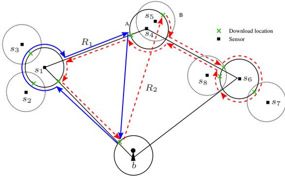
Fig. 4. Division of a TSPN tour into 2 subtours using DGP algorithm.
