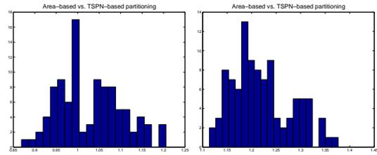
Fig. 8. The histograms shows the ratio of the coverage time of an area-based partitioning algorithm to the coverage time of the TSPN-based partitioning algorithm. **Left:** In this case the sensors were deployed uniformly at random, and the performance of the two algorithms was comparable. **Right:** In this case the sensors were deployed non-uniformly (See Figure 10) and the TSPN-based partitioning approach clearly outperformed the area-based approach.
