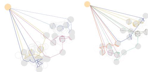
Fig. 10. **Left:** Data gathering using an area-based partitioning approach. **Right:** Data gathering using a TSPN-based partition. In this instance, TSPN-based partitioning was 37% better. In both figures, gray disks correspond to the disks in MIS. The base station is the yellow disk on the top left.
