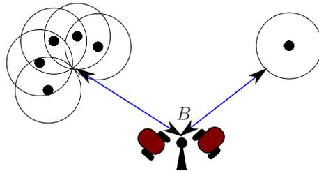
Fig. 1. Two robots charged with collecting data from the sensors and relaying them to the base station  $B$ . The filled circles correspond to sensor locations. The circle around a sensor illustrates its communication range. The figure shows optimum TSP tours for the two robots which minimize the maximum travel distance by any robot. This solution is not appropriate for data gathering because the robot assigned to the left group would spend a lot of time downloading the data from the sensors.
