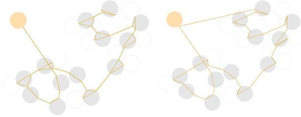
Fig. 6. Data gathering tours for a single robot based on **Left:** TSPN\_TOUR (the total coverage time is 4044 units), **Right:** ONE\_WAY\_TSPN\_TOUR (the total coverage time is 2765 units). In this instance, the proposed modification yields significant improvements. In both figures, gray disks correspond to the disks in MIS. The base station is the yellow disk on the top left.
