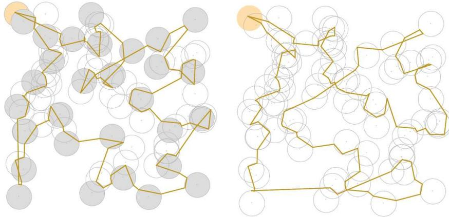
Figure 9: An instance where the DGP tour performs better than the k-TSP tour of download locations by 15%. Transmission range of the sensors is 40. The base station is the top left disk in yellow (lighter) shade in both the figures. **Left:** Data gathering with one robot using *DGPTour*. **Right:** Data gathering with one robot using k-TSP tour of download locations.
