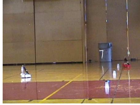
(b) A snapshot from the experiment with two mules. One mule (white robot) is following its designed path while the other mule (red robot) is downloading data from the assigned mote.
