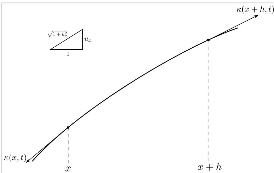
Figure 2: Balancing forces to derive the wave equation
