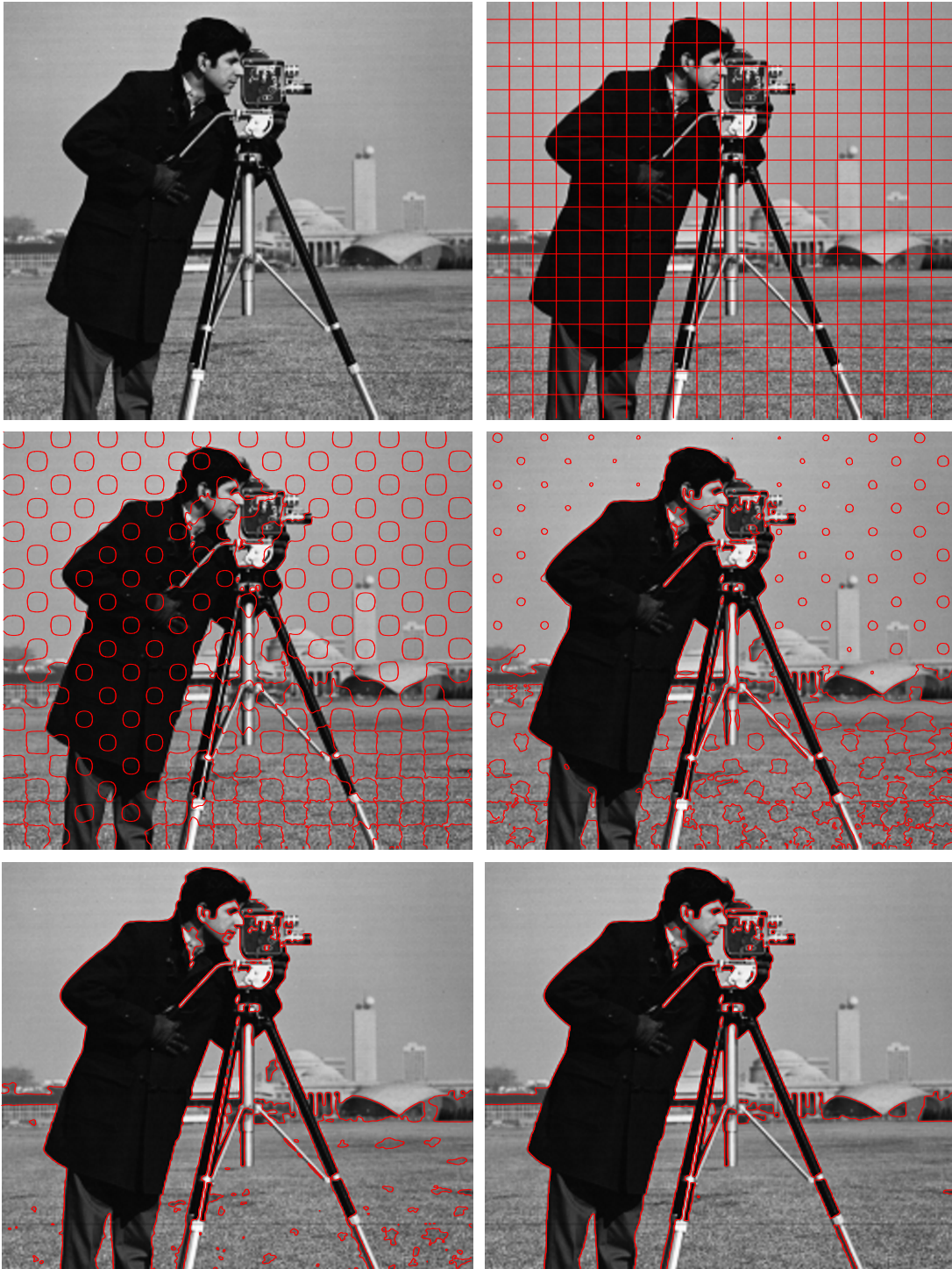
Figure 3.8: Illustration of gradient descent for segmenting the cameraman image. Top left is the original image, and top right is the initialization of the gradient descent algorithm. The lower four images show the evolution of the zero level set of u .
