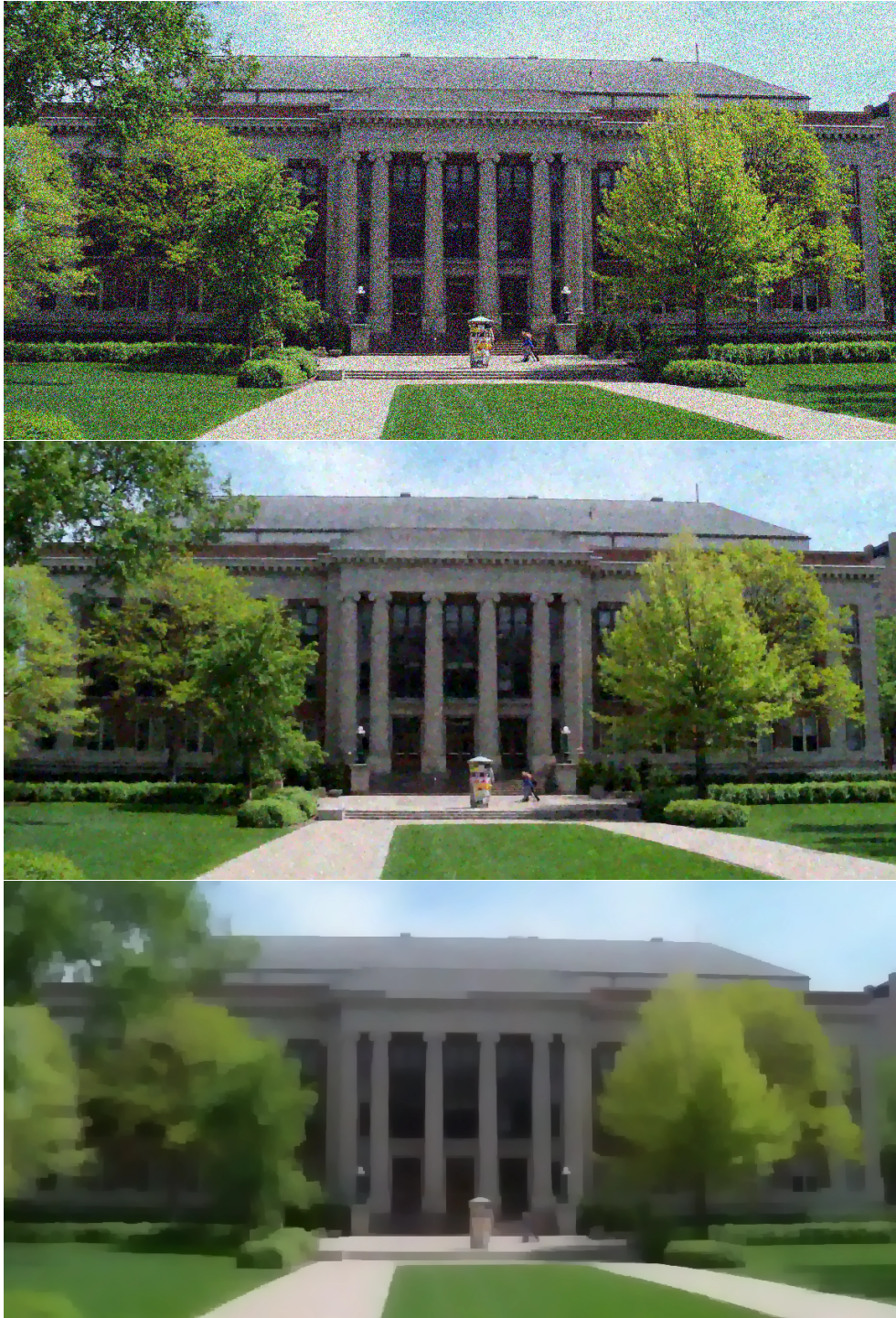
Figure 3.7: Example of TV image restoration: (top) noisy image (middle) TV restoration with small value for \lambda , and (bottom) TV restoration with large value for \lambda .
