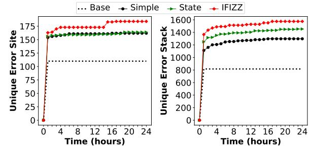
Fig. 6. Code coverage of different fault-scenario generation approaches.
