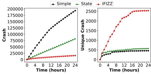
Fig. 5. Crashes discovered by different fault-scenario generation approaches.
