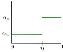
$$R \frac{\partial T}{\partial t} = Qs(y)(1 - \alpha(y, \eta)) - (A + BT) - C(T - \bar{T})$$
