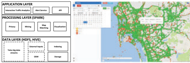
Figure 2: (Left) The components of the proposed Traffic-TBD architecture. (Right) A preliminary version of the spatio-temporal Traffic-TBD analytic interface.
