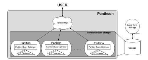
Fig. 1. Pantheon System Architecture
