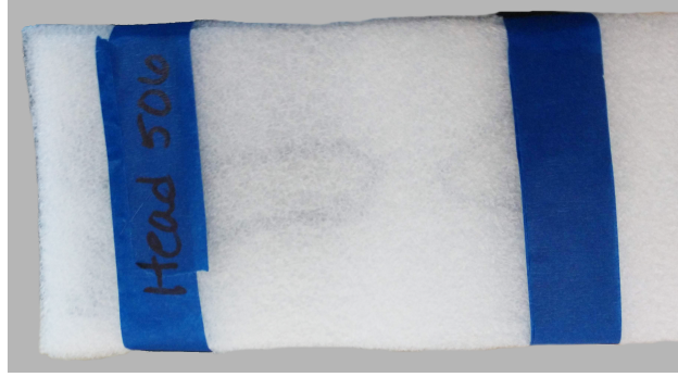
Figure 5: Pictured here is an example of how we labeled the package indicating how to orient the package on the scanning bed and as a cross-reference for the .csv file for that scan package.
