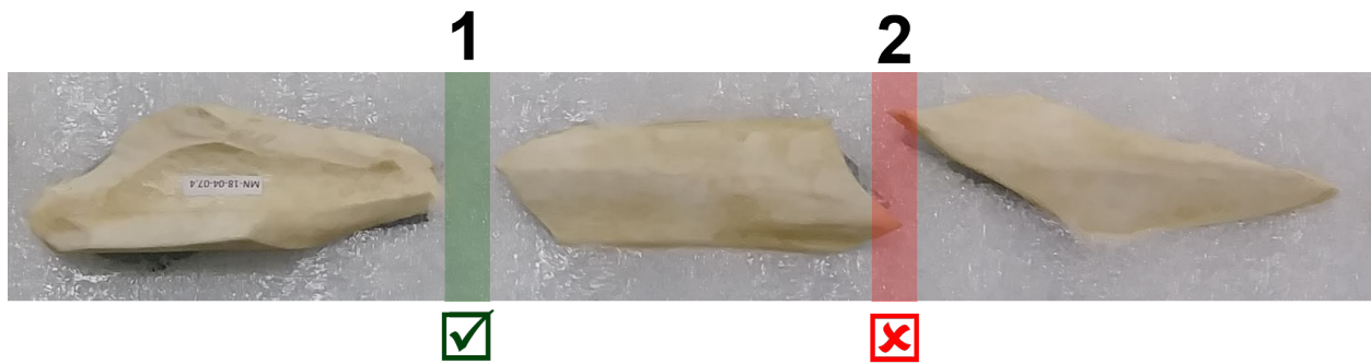
Figure 2: Fragment placement: The fragments should not overlap in the x - or y - directions. This ensures that the automated segmentation can properly separate the fragments within the scan data into individual models for surfacing. The x -axis is the view from the side of the scanning bed. The y -axis is the bird's eye view of the scanning bed.
