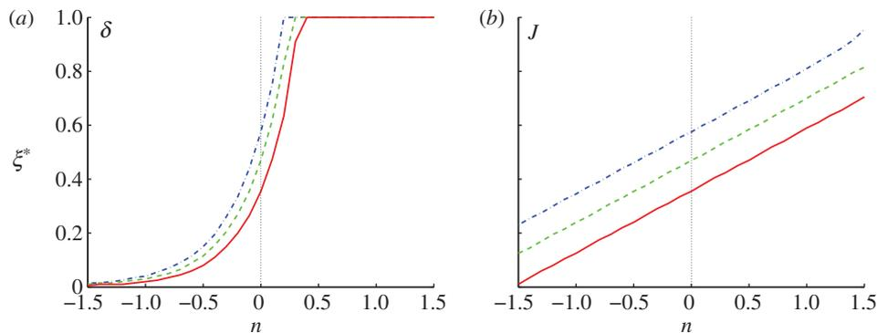
Figure 11. The variation of the boundary locations as the flux and dimensionless diffusion coefficient are varied in the stochastic version of scheme I. The  $y$ -axis is the compartment number normalized by 200 and the  $x$ -axis indicates the variation of the parameters. (a)  $\delta = 10^{n-1}$ , (b)  $J = 10^{3+n}$ .
