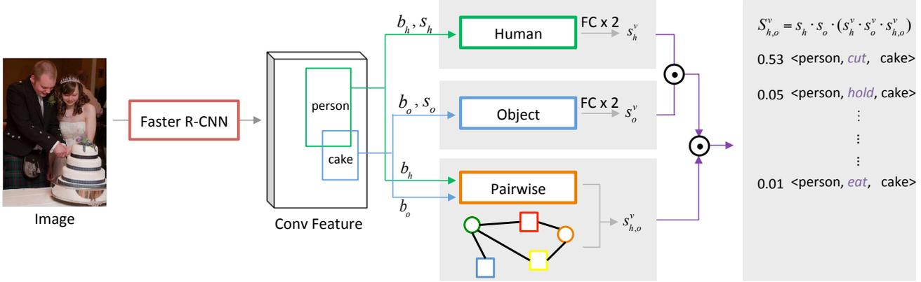
Figure 3: The inference procedure of the proposed model. Given an input image, the proposed model detects HOI triplets and outputs the triplet scores. Element-wise multiplication ( $\odot$ ) is applied to human stream’s verb prediction  $s_h^v$ , object stream’s verb prediction  $s_o^v$  and the pairwise verb prediction score  $s_{h,o}^v$ .
