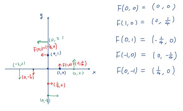
One can think such a vector field represents fluid flow in 2 dimensions. Thus F(x, y) gives the **velocity** of a fluid at the position (x, y). We call F(x, y) the **velocity field of the fluid**.
