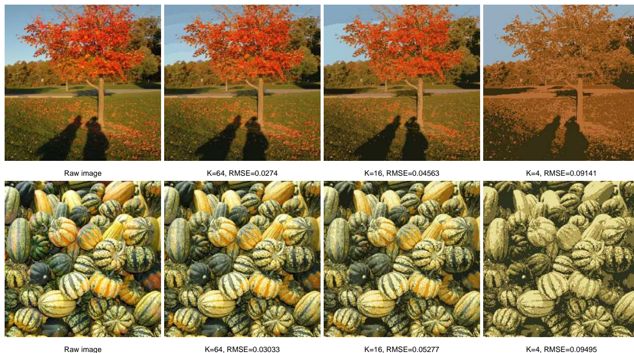
Figure 11: Results of color clustering by FCDC. First column: raw image; second column: 64 colors; third column: 16 colors; last column: 4 colors.
