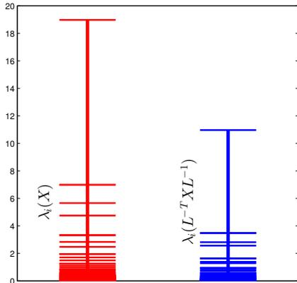
FIG. 3.1. *Illustration of the decay of eigenvalues of  $X$  (left) and  $S^{-1} - C^{-1} = L^{-T} X L^{-1}$  (right) for a 2-D Laplacian matrix with  $n_x = n_y = 32$ , where the domain is decomposed into 4 subdomains (i.e.,  $p = 4$ ), and the size of  $S$  is 127. 5 eigenvectors will capture 82.5% of the spectrum of  $X$  and 85.1% of the spectrum of  $L^{-T} X L^{-1}$ , whereas 10 eigenvectors will capture 89.7% of the spectrum of  $X$  and 91.4% of the spectrum of  $L^{-T} X L^{-1}$ .*
