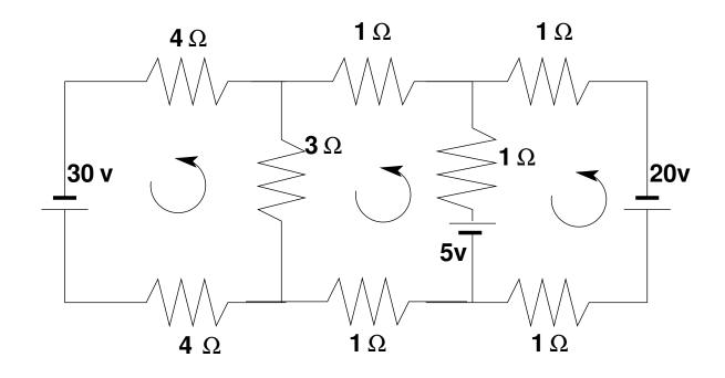
Problem: Determine the loop currents in a an electrical circuit - using Kirchhoff's Law (V=RI)
